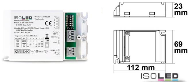
**111989** | LED MULTI Trafo 12V/24V/350mA/500mA/700mA, Push + 1-10V dimmbar, SELV
